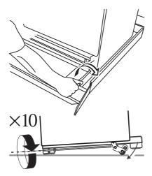
Make sure you lower BOTH REAR ROLLERS. There are two adjusting nuts, one for each roller, at both the front bottom corners of the cooker. Open the grill door and the Holding oven door. Grip under the facia panel and lift the front of the cooker.
